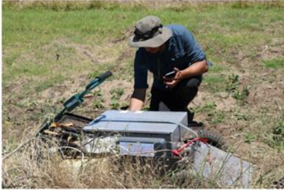
Image: Microwave applicator prototype trial on Skeleton weed in Munster (Source: DPIRD)
