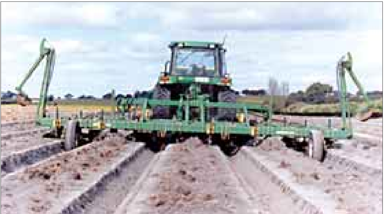
Figure 28. Rear view of a 3-point linkage bed-former. Note the gauge wheels, bracketed attachments, grader blades, half beds at either extremity of the bar, marker arms and square shoulders of the beds.
