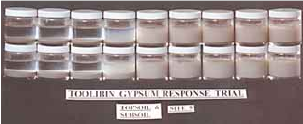
Figure 14. Gypsum response test on the soil from a Raised Bed site at Toolibin. Soil is mixed with distilled water (right) and progressively increased gypsum solutions (left). The concentration of gypsum solution at which clay flocculates (suspension settles) is converted to tonnes of gypsum/ha/depth of soil.
