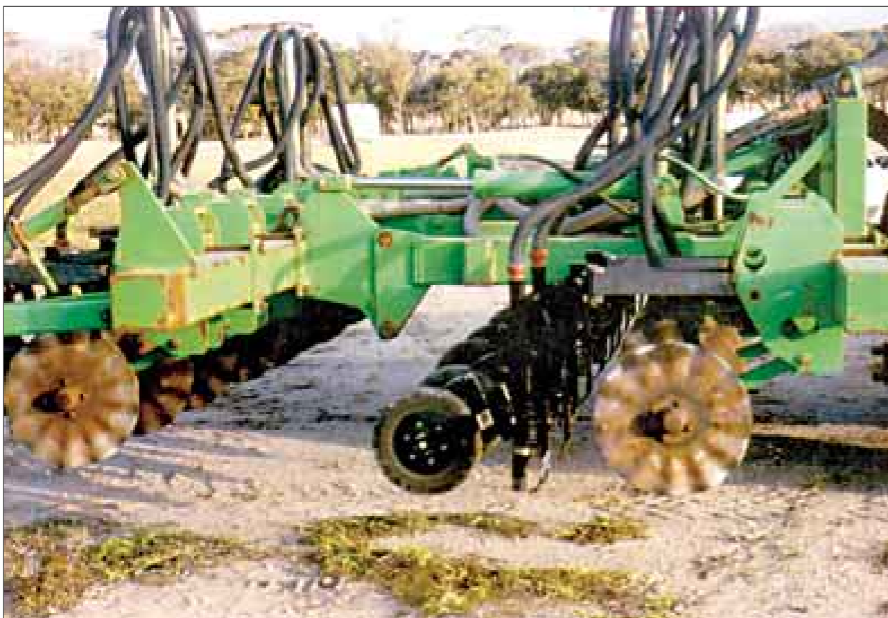
Figure 33. View of our hybrid seeder specially set up for seeding Raised Beds. Note the wavy coulters and parallelogram seed placement and press wheel assembly.
