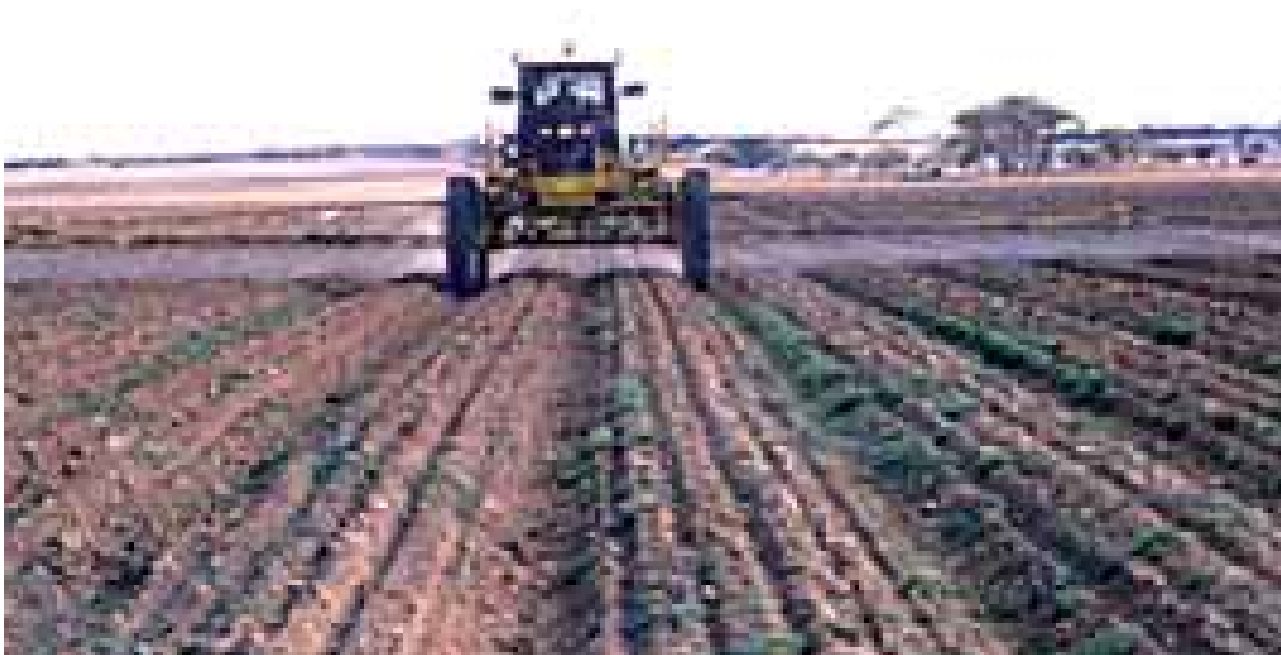
Figure 36. View of a self-propelled sprayer in Raised Beds. Note that the track width of this 90ft boom spans two beds and has 6 beds on one side and 7 beds on the other. Six feet (one bed width) of the boom was shut-off so the boom covered 6 beds each side of the tank and cabin.
