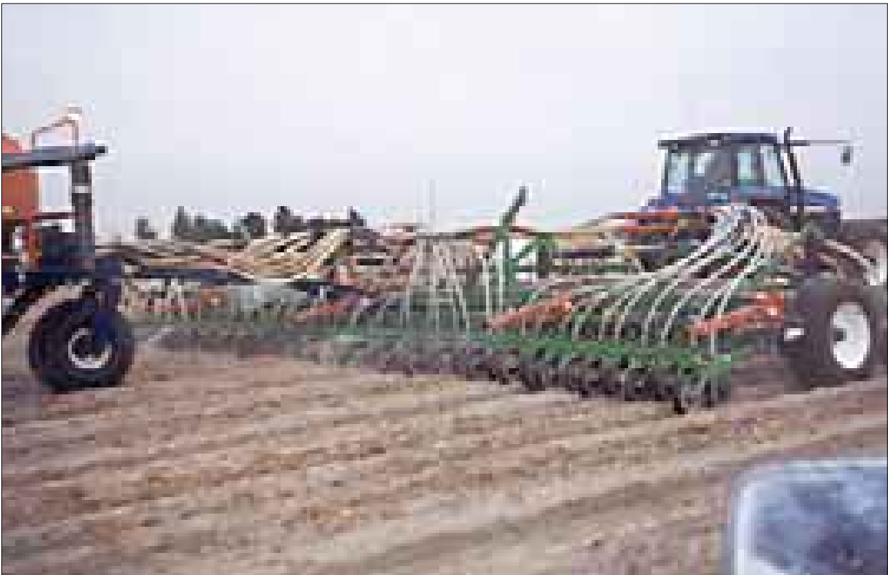
Figure 35. A farmer's Raised Bed seeder. The bar was specially built to fit the beds. It has triple disc seeder units. The air-seeder has not been adapted to fit the furrows. It tracks on top of the beds.
