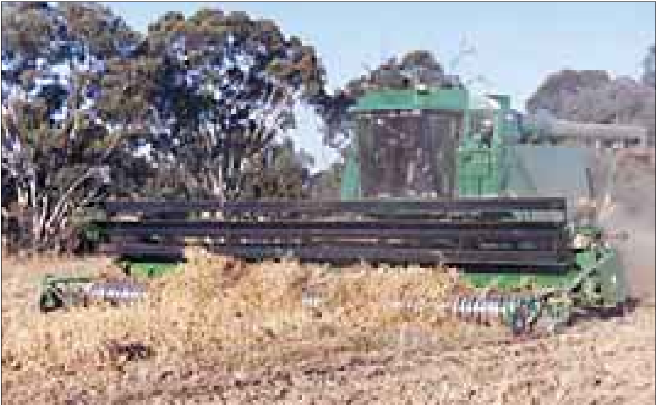
Figure 42. Converted harvester in a pea crop at Woodanilling. Note that the pea vine is being easily lifted.
