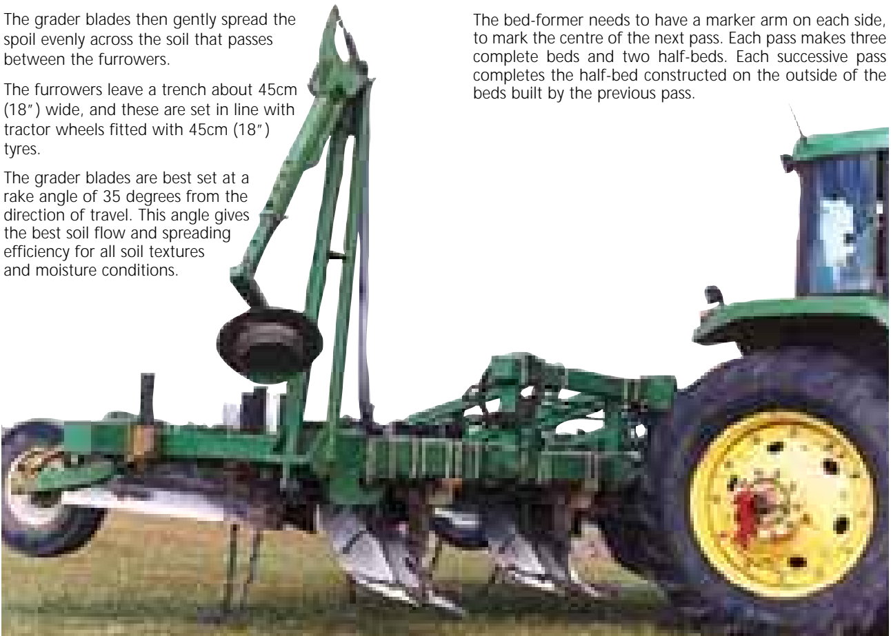
Figure 16. View of bed-former showing the scour pattern produced on the furrowers and grader blades indicating the machine has been properly set up.
