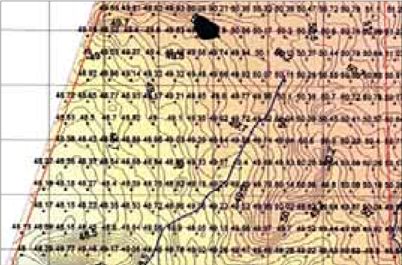
Figure 6. An example of a high precision contour survey done for planning the layout of Raised Beds and drains at Badgingarra. The map shows 10cm contours and spot heights of grid points. This was produced by DGPS technology.
