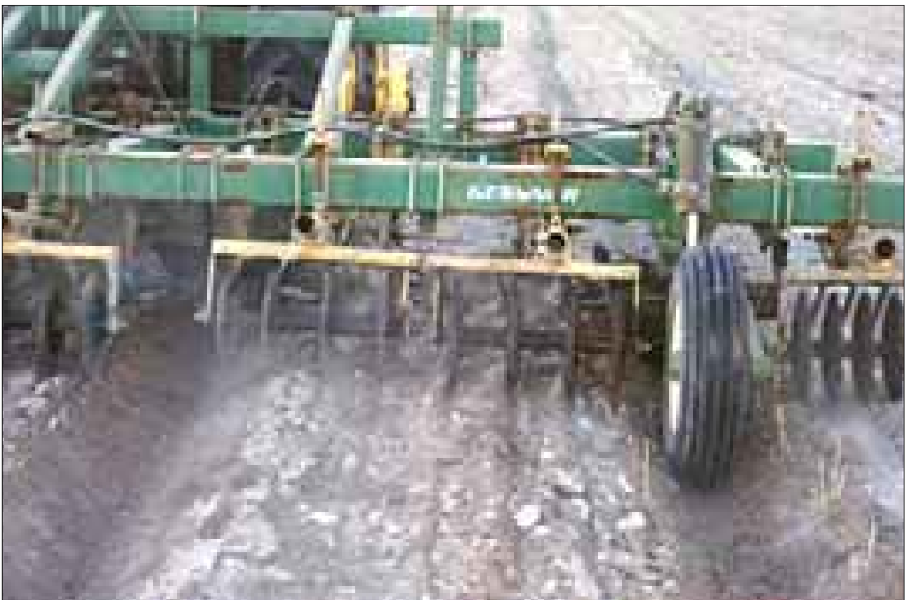
Figure 31. Rear view of a bed-former renovating beds. Note suspended disc harrows breaking the soil crust and the looseness of the beds from shoulder to shoulder
