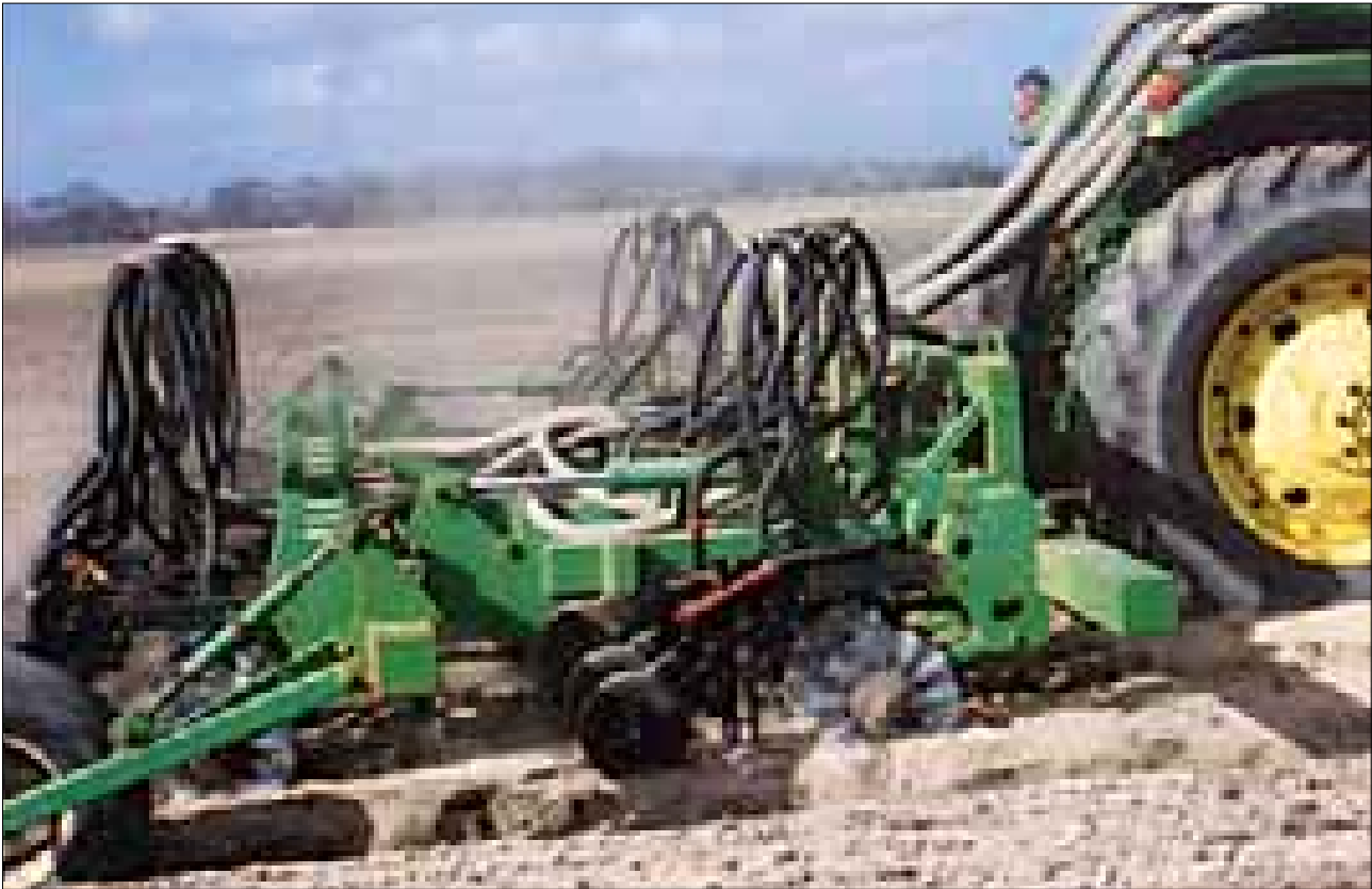
Figure 34. The hybrid seeder operating in raised beds at Woodanilling. Note the retention of the shoulder during seeding.
