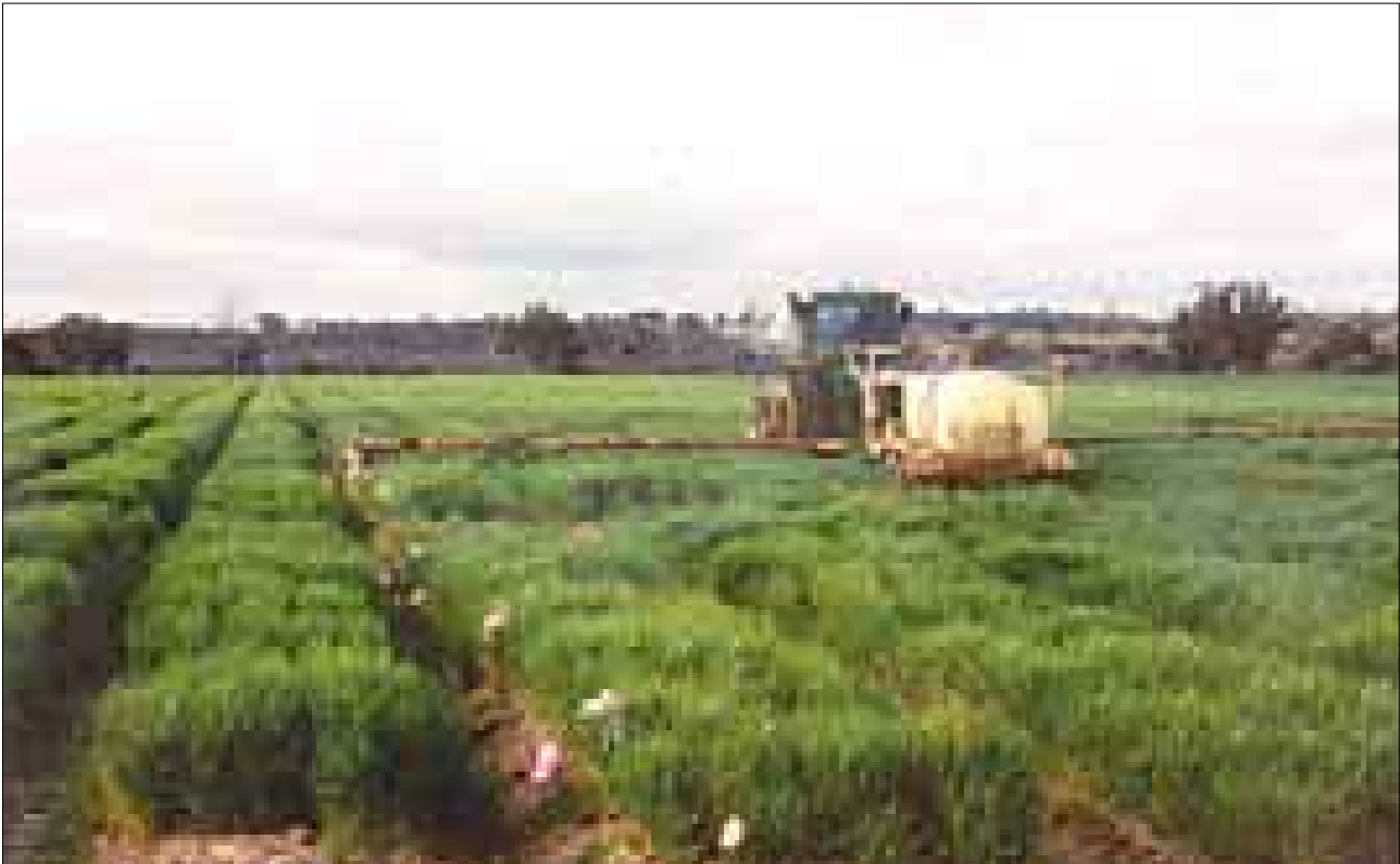
Figure 37. A towed spray tank in beds at Woodanilling. Its trackwidth is compatible with the 1.83m bed spacing.
