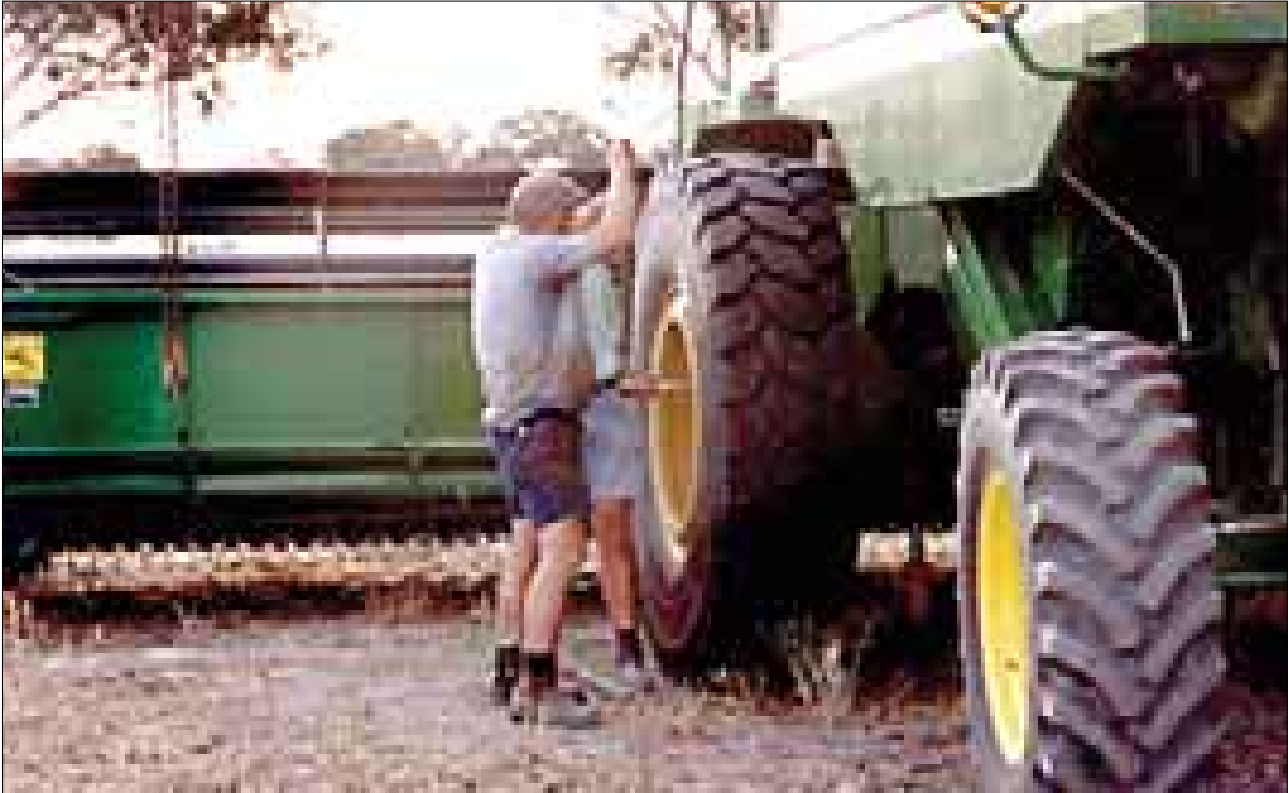
Figure 40. Fitting 18" dump truck wheels to a John Deere 9600 harvester in the paddock. Note the position of the mounting disc inside the rim and the alignment of the driving and steering wheels.
