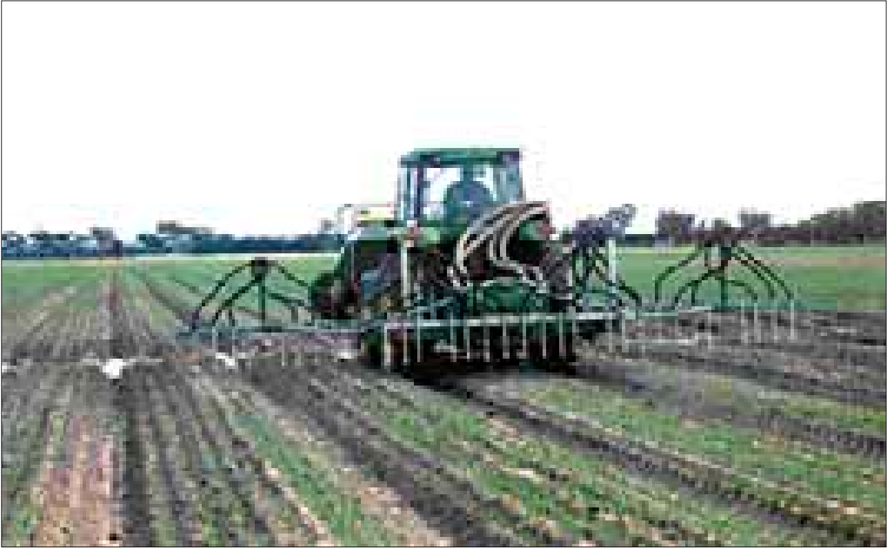
Figure 38. View of a fertiliser bar that makes use of the air seeder (tractor mounted in this case) for applying mid-season fertiliser dressings with high precision in Raised Bed crops.
