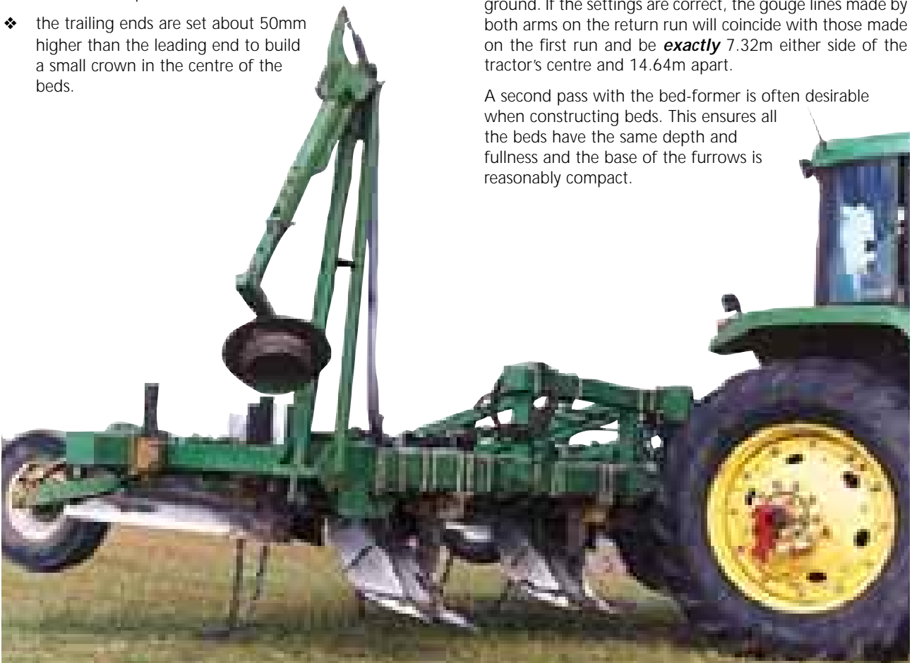
Figure 29. Side view of bed-former showing the positioning of components and scour patterns on furrowers and grader blades indicative of a properly set up machine.
