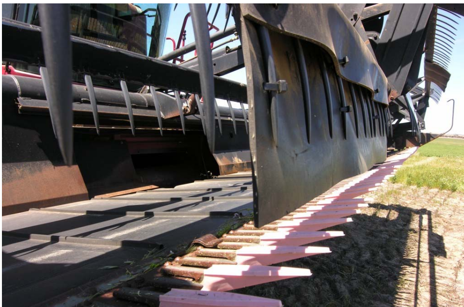
Figure 2 Primary Sales Adapter-Gap pink extension fingers and rubber sweeps on reel.
