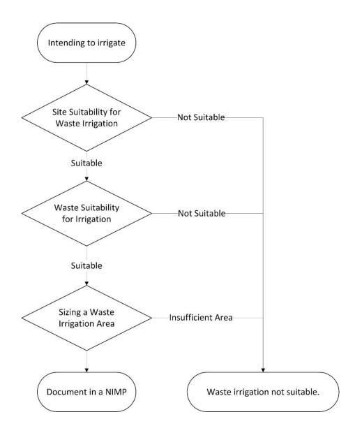
Once the environment and liquid waste are deemed suitable for irrigation, the following steps can be taken to size a waste irrigation scheme:
