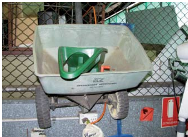
Before storage, fertiliser needs to be removed from spreader.
