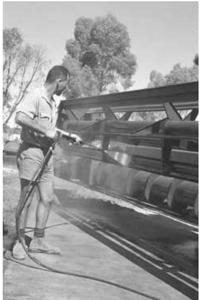
Cleaning harvesters between paddock movements will reduce weed spread on the property
