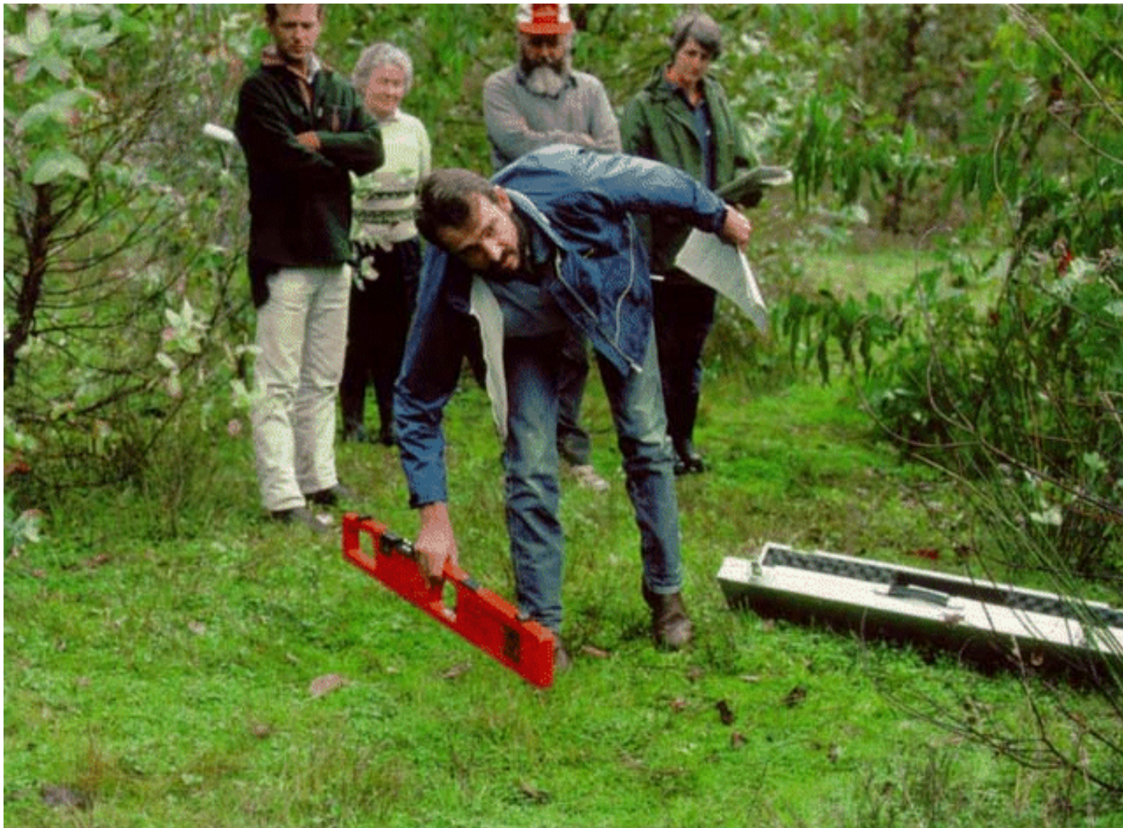
Figure 2. Don Bennett using an EM/38 to measure soil salinity
