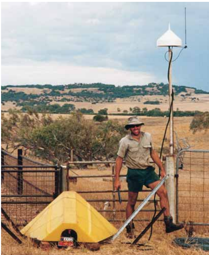
Photo 6.3 Base station located on-farm to achieve +/- 1-2cm accuracy with a DGPS auto-steer guidance system. Check the manufacturer's recommendations for the ideal position relative to the working area.
