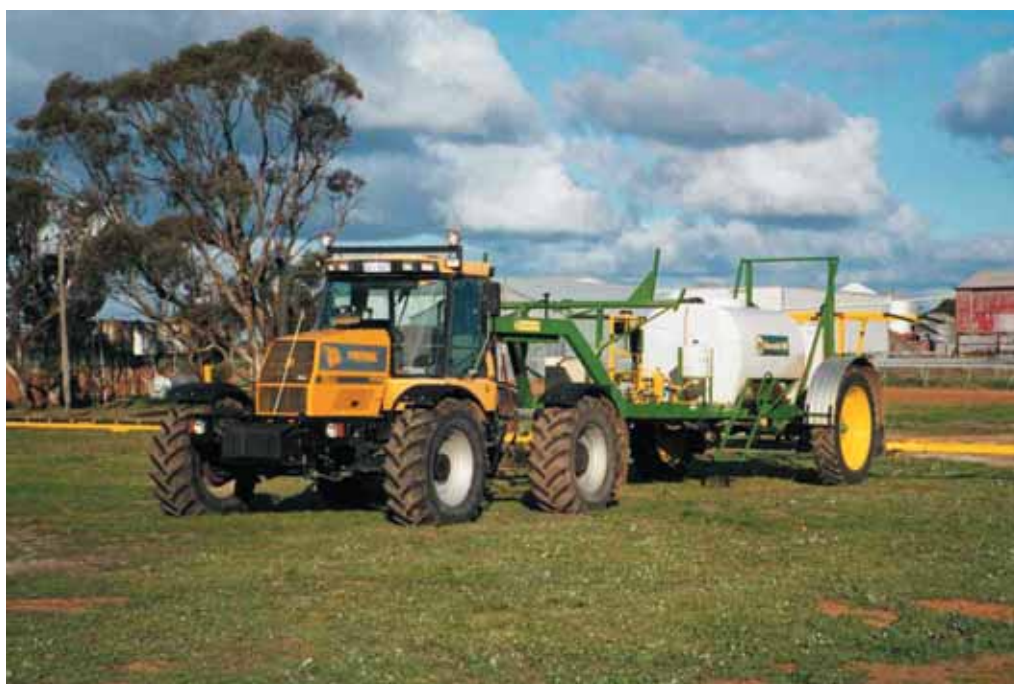
Photo 11.13. Owen's JCB with modified axles to 3m towing a boomspray with adjustable axles.
