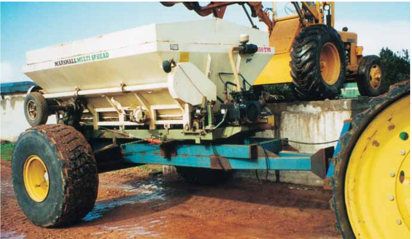
Photo 7.3 The spreader has been mounted on an old truck axle modified to a 3 m track. Modifications to vehicle axles may require risk assessment on-farm and re-certification for road use.
