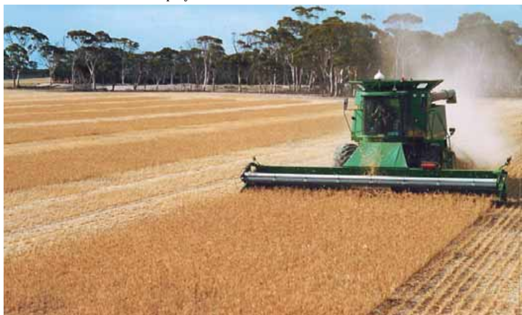
Photo 11.10. Fretwell's harvester on auto-steer.
