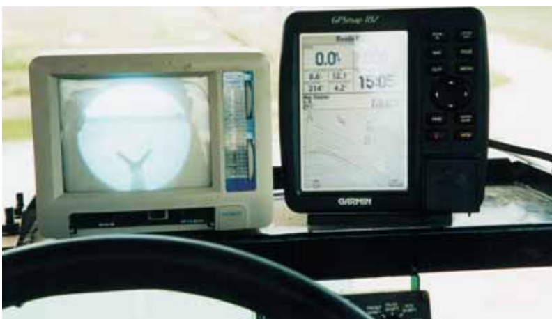
Photo 6.2 A video camera located on the wing of the air seeder bar (a) is used to record an image displayed in the tractor cab (b) on the left.
