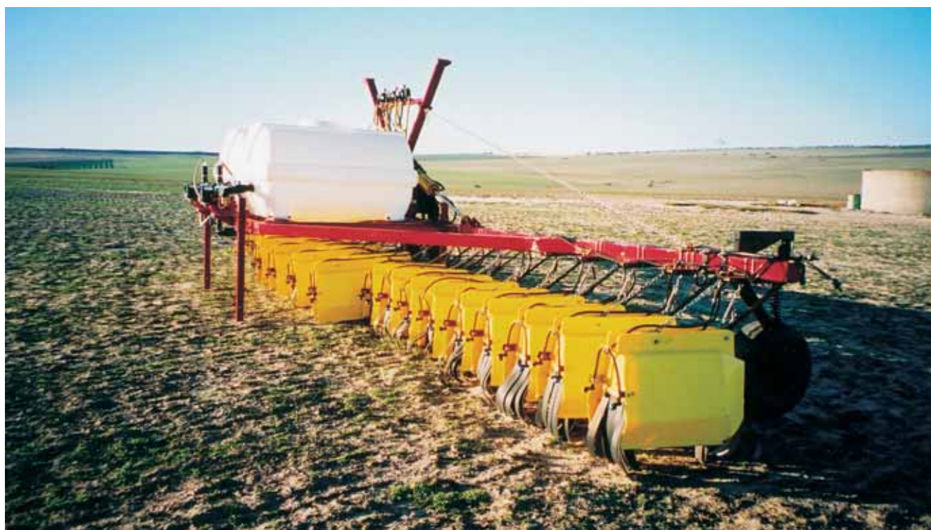
Photo 11.6. Obst's inter-row shielded sprayer.
