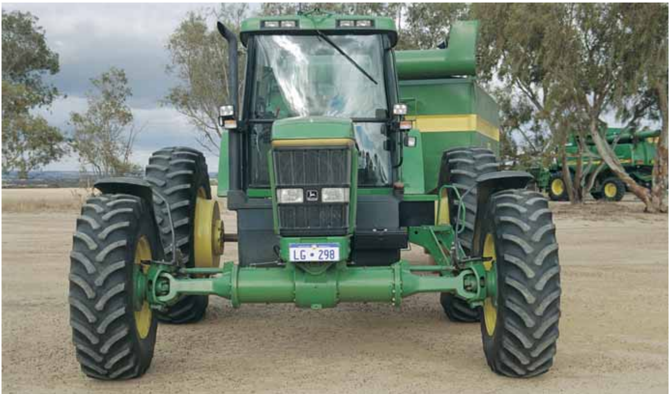
Photo 7.2 This John Deere tractor has had the front axle extended to 3 m centres
