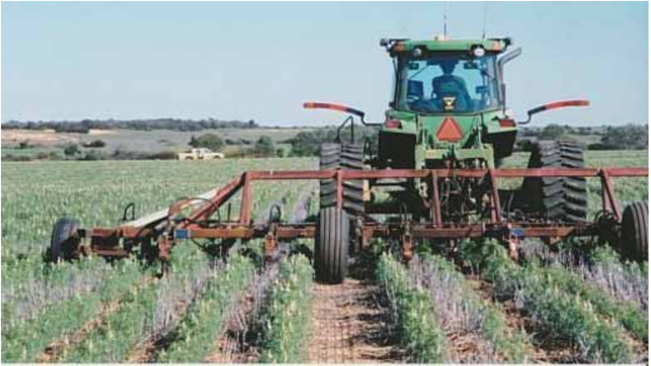
Photo 11.9. Deep ripping between lupin rows during flowering
