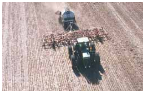
Photo 11.4. Paddy seeding in 2002 up and back with dGPS auto-steer.
