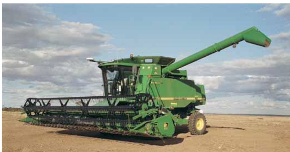
Photo 7.6 Extended auger on a John Deere harvester with a 9.1 m front to enable unloading into a chaser bin on adjacent tramlines
