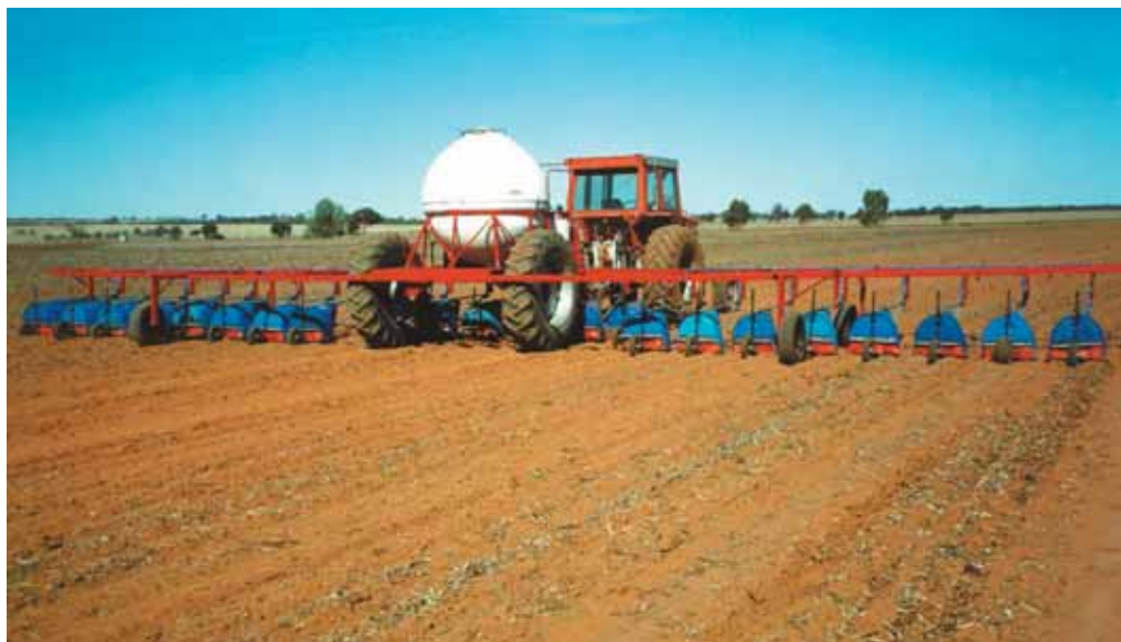
Photo 10.6. Self-steering shields made by Harold and Glenn Millington, Burracoppin, from on-farm materials.
