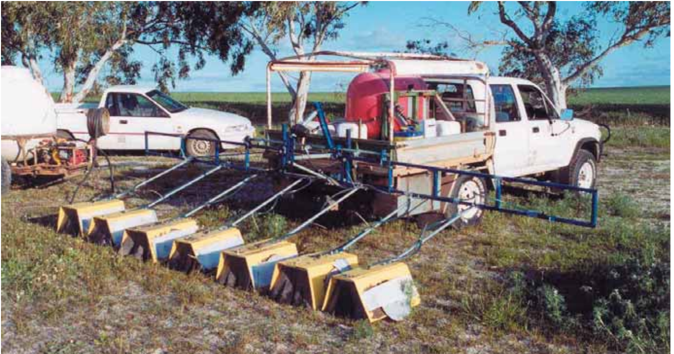
Photo 10.4. The setup used for the Rowcrop Rocket designed by Mike Collins mounted on a spray ute in 2002. The shields are set up the same distance behind the hitch point as the ute axle is in front. As a consequence, when the ute turned to the left, the ute rear swings to the right, helping to compensate for the tendency for the shields to cut the corner.
