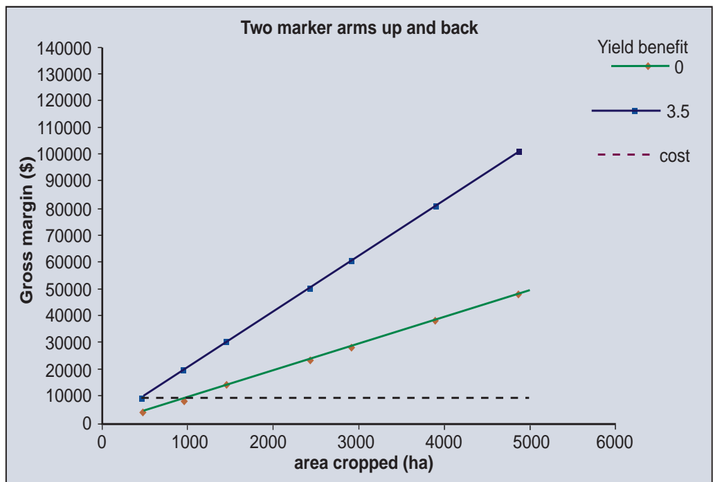
Figure 1.5. Estimated economic benefits of two marker arms working up and back. Gross margins are based on 2 t/ha yield, $150/t on-farm price, $60/ha fertiliser cost and $40/ha herbicide cost. Ten per cent input reduction. Yield benefit zero per cent equals overlap savings only; 3.5 per cent equals matching tracks and mechanical guidance.
