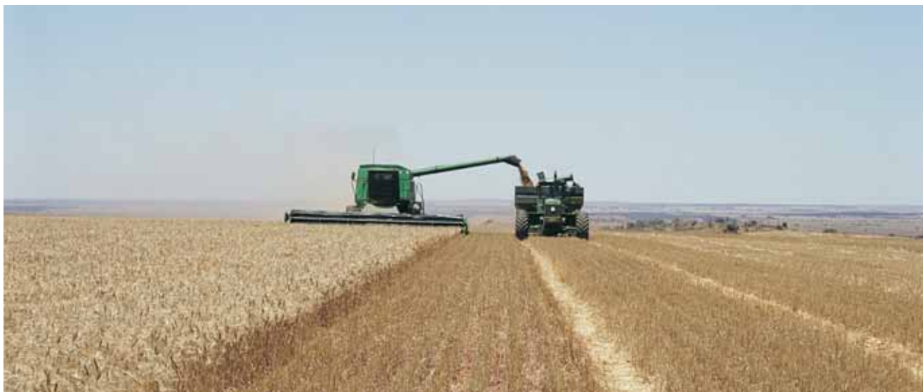
Photo 7.5 Unloading on adjacent tramlines with a 9.1 m harvester front.
