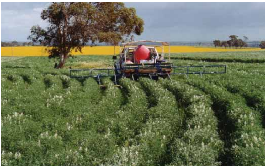
Photo 10.5. The setup for Rowcrop Rockets mounted on a spray ute on a 40m radius curve. This is about the maximum angle for this setup.
