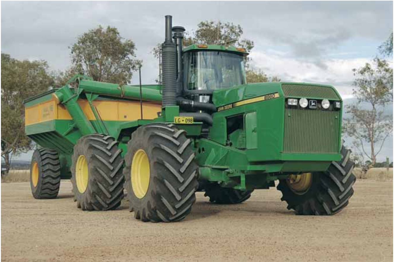
Photo 11.11. Fretwell's seeding tractor pulling the chaser bin with a matching 3m wheel track.
