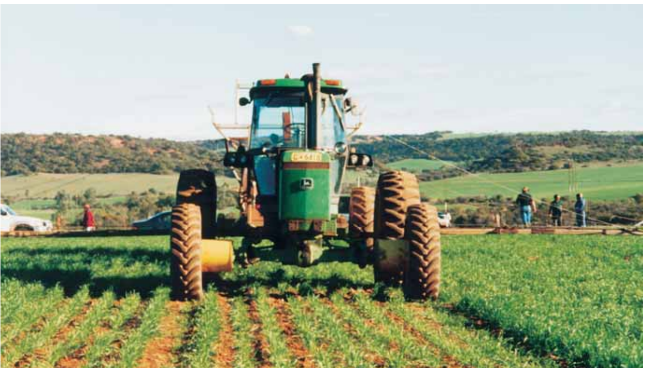
Photo 7.1 Cotton reels have been used to take the John Deere JD4250 MFWD tractor axle out to 3 m
