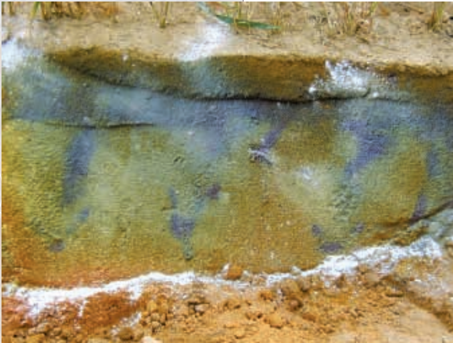
Figure 2: Cutaway soil profile over the top 20 cm of soil. The profile was treated with pH indicator solution and pH indicator powder. Note the purple areas that show where the lime has been placed during subsurface liming.
