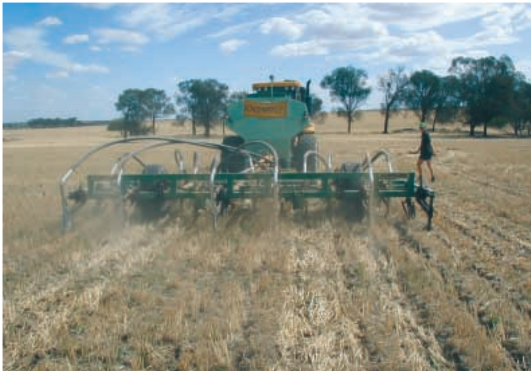
Figure 3: Deep ripping and placement of lime at depth using grower scale machinery at Corrigin.
