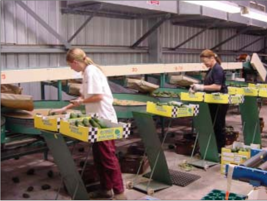
Figure 14. Packing of avocado fruit into trays after a weight grader has sorted the fruit into size groups.
