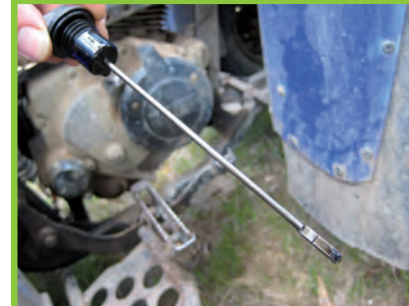
Periodically check engine oil level (above) and radiator coolant level if the ATV is liquid cooled. Only check coolant level on a cold engine.
